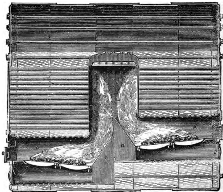
Vertical longitudinal section of one of the nine boilers of the "Alaska."
